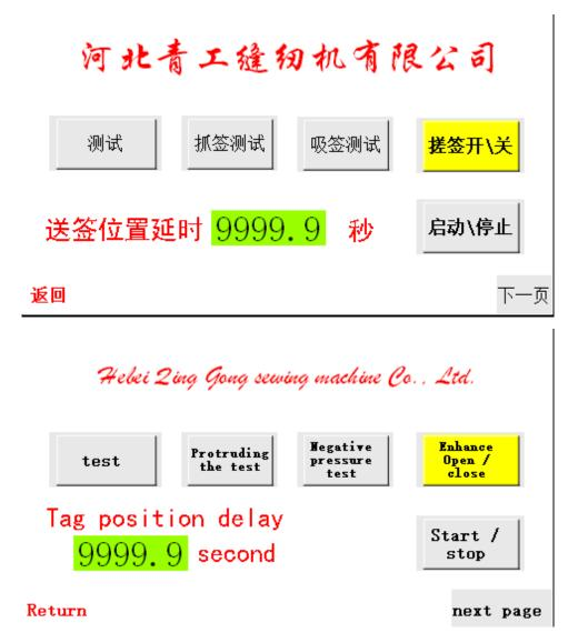
(1) **Start/Stop button**: Press the start/stop button, the labeling machine to start automatic positioning. After the positioning is completed, the robot grabs a label and waits for the arrival of the bag to prepare the label.
